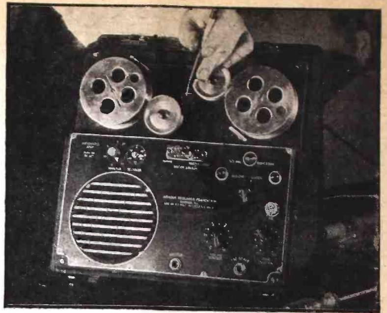
Courtesy Armour Research Foundation The new magnetic recorder. Wire reels are plainly visible, and pencil points out the recording head through which the wire runs.
